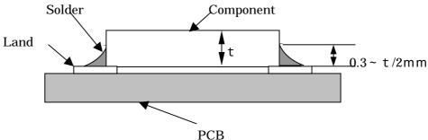
Example) When a 0.3 mm thick solder mask is used, fillets will be about 0.95 mm
